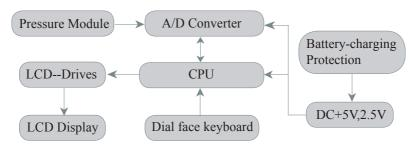
Apply pressure to the pressure transducer, it outputs a electrical signal. First the corresponding electrical signal will be amplified and then it will be converted to digital data by A/D converter. Then the microprocessor sequentially collects data to modify and correct, the final result will be displayed on the LCD Display.
